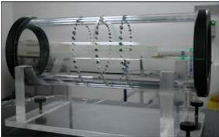
Geometry Calibration Phantom
