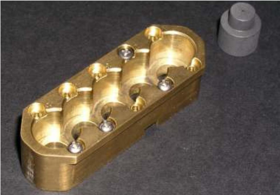
Graphite Target and Electron Substrate
